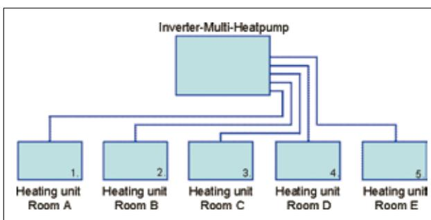
Figure 3. Inverter heat pump can serve up to five indoor units
