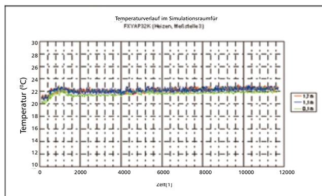
Figure 1. Temperature variation in room equipped with inverter heat pumps
